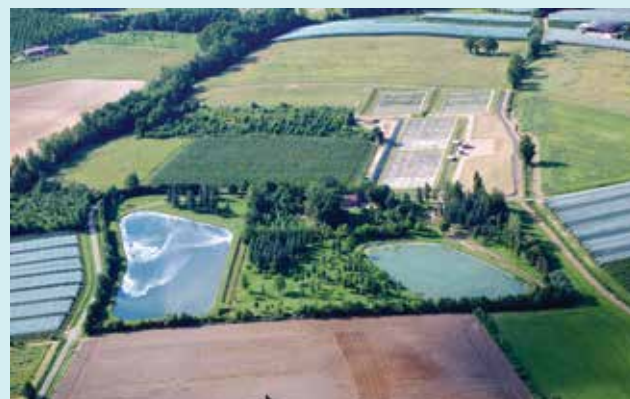
AN AERIAL VIEW OF THE PLANT: TOP, THE 2 LAGOONS, BOTTOM LEFT, THE 2 FILTER STAGES
