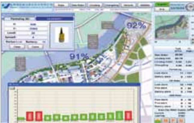
Daily monitoring of data returned by the acoustic leak detectors
