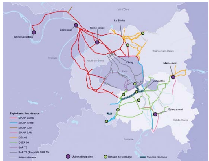
Figure 1: Sanitation system under SIAAP project management
